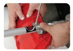
2b. Tighten the screws after setting the safety cover bracket at the appropriate position.
