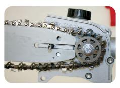
**8c.** Place the chain around the bar. Make sure that the cutting teeth face the front.
