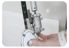
9. Install the hedge trimmer. Find the longer spline end and place the end to the hedger. Tighten it.
