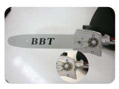
8b. Place the chainsaw bar in its place. Turn the bar adjuster all way in, to let the bar sit on the wheel.
