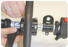
1a. Position the handle in a comfortable operating position and tighten the screws.
