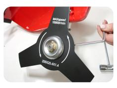
7. Install the brush cutter. Remove the outer holder (see step 3). Place the blade and outer holder back to the position. Lock the inner holder with Allen Key and turn the nut anti-clockwise.
