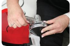
5. Install the line. Insert the line in the hole and push it forward until the end comes out 2-3 cms from the other hole.
