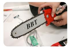
8e. Place the cover back. Adjust the bar adjustment to set the chain in the desired tension. Tighten up again before every use.
