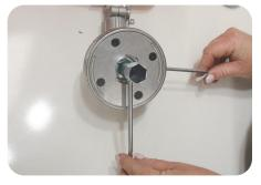
4. Install Line Trimmer. Align the hole in the adapter plate with the hole in the shaft and install it with the lock tool. Rotate the nut anti-clockwise until it is securely tightened.
