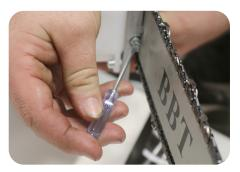
8d. Unscrew the bar adjustment to set the chain in the bar.
