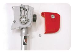
8. Install the chainsaw bar and chain. Remove the screw on the cover and take off the cover.
