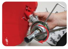
3. Install the Brush Cutter / Line Trimmer. Remove the outer holder. Insert the Allen Key to lock the inner holder and rotate the left-handed thread nut in the clockwise direction.
